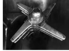
Figure 3.12: Knife head of resinating mixer
