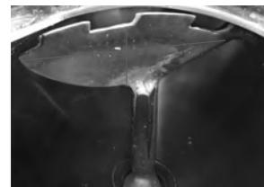
Figure 3.11: Mixing arm type II of resinating mixer
