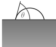
Figure 3.3: Schematic depiction of contact angle  $\theta$
