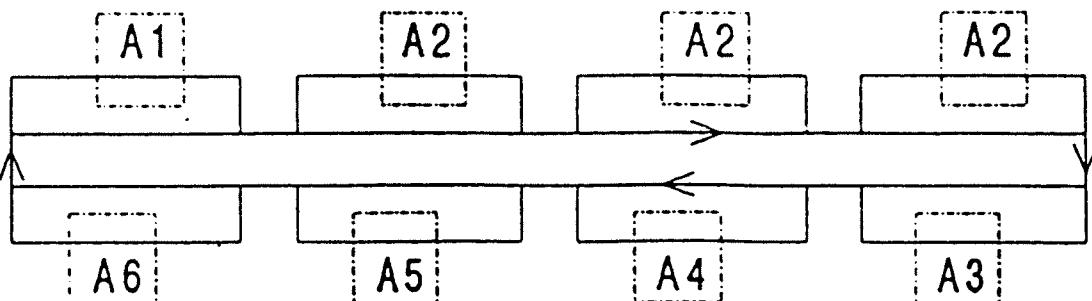
Two parallel conveyor belts, B1 and B2, are linked together at both ends. An assembly station Ax is placed at B2. Pallets are coming in on belt B1. If they are to be processed in Ax they are shifted in Sx to B2 and possibly enter a queue in front of Ax. If there is no more empty buffer space on B2 or the pallet is not to be processed in Ax it continues its way along B1. Parts that have been processed in Ax are shifted back to B1 in Sy, having priority over those coming from the left on B1.
