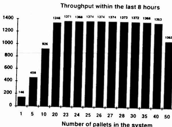
The system has its maximum throughput for 25 - 27 pallets. The respective cycle times are given in the following diagram:
