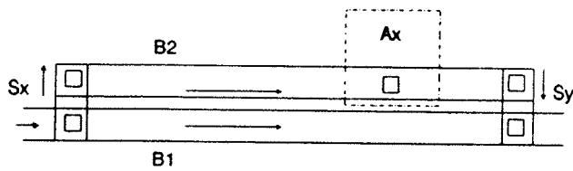
Two parallel conveyor belts, B1 and B2, are linked together at both ends. An assembly station Ax is placed at B2. Pallets are coming in on belt B1. If they are to be processed in Ax they are shifted in Sx to B2 and possibly enter a queue in front of Ax. If there is no more empty buffer space on B2 or the pallet is not to be processed in Ax it continues its way along B1. Parts that have been processed in Ax are shifted back to B1 in Sy, having priority over those coming from the left on B1.
