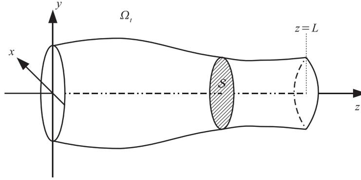
Figure 1: Schematic representation of a vessel segment as cylindrical tube
