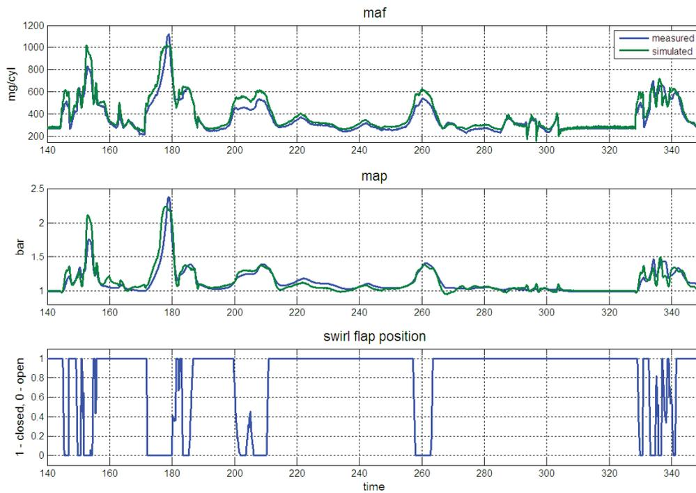
**Figure 4.** Overall model performance during swirl valve operation
