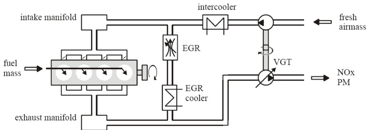
Figure 2 Scheme of the air path of a turbo charged Diesel engine
