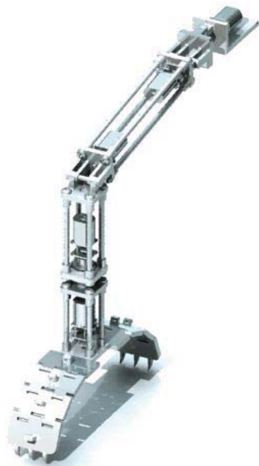
Figure 2: Kamanbaré leg - kinematic configuration.
