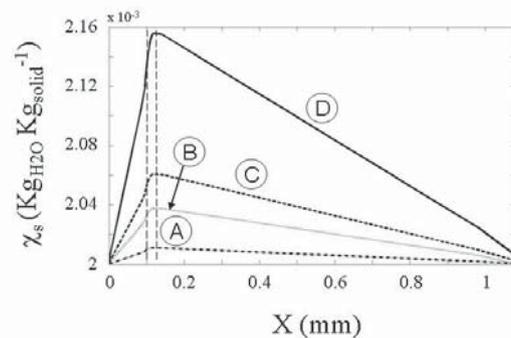
**Figure 13:** Steady-state spatial distribution of liquid water.  $J_e = 0.119 \text{ A}\cdot\text{cm}^{-2}$  (A),  $0.404 \text{ A}\cdot\text{cm}^{-2}$  (B),  $0.650 \text{ A}\cdot\text{cm}^{-2}$  (C),  $1.643 \text{ A}\cdot\text{cm}^{-2}$  (D).
