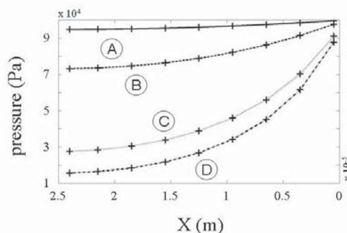
**Figure 14:** Steady-state partial pressure of  $O_2$  along the catalytic layer corresponding to different current densities:  $0.069 \text{ A}\cdot\text{cm}^{-2}$  (A),  $0.413 \text{ A}\cdot\text{cm}^{-2}$  (B),  $1.744 \text{ A}\cdot\text{cm}^{-2}$  (C),  $2.487 \text{ A}\cdot\text{cm}^{-2}$  (D).
