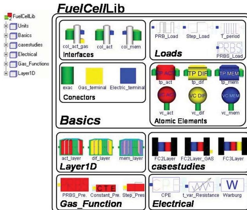
Figure 1: Packages and models of *FuelCellLib* 2.
