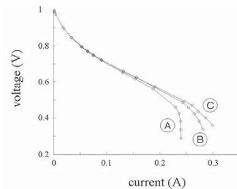
**Figure 9:** Polarization curves. Partial pressure of oxygen at the cathode:  $p_{O_2} = 1$  atm (A),  $2$  atm (B),  $3$  atm (C).
