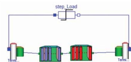
**Figure 5:** Experimental setup to study the cell response to a step change in load.
