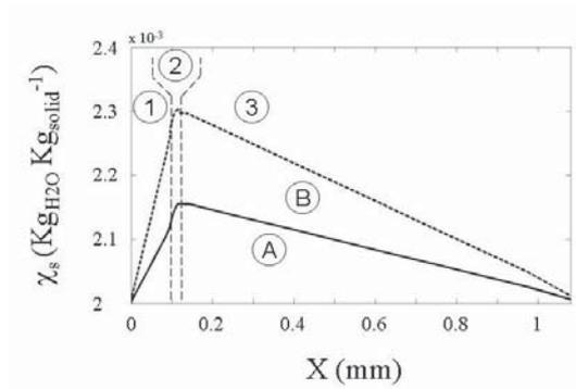
**Figure 10:** Water load along the spatial dimension: membrane,  $10^{-4}\text{m}$  (1), catalytic layer,  $2.5 \cdot 10^{-5}\text{m}$  (2) and diffusion layer  $10^{-3}\text{m}$  (3). Without (A) / With (B) electro-osmotic drag.
