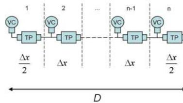
Figure 2: Spatial discretization of a layer.
