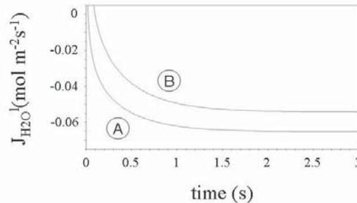
**Figure 11:** Flow of liquid water in the center of the membrane. Without (A) / With (B) electro-osmotic drag.
