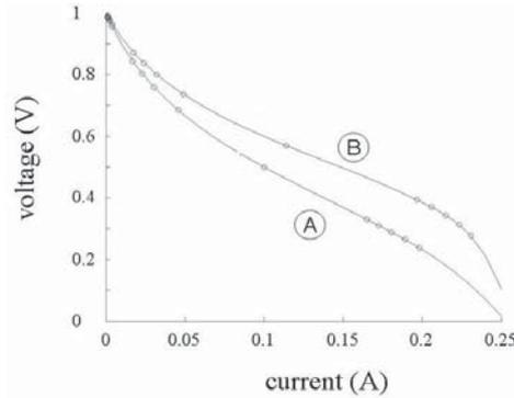
**Figure 7:** Effect of the Tafel slope ( $b_T$ ) on the polarization curve.  $b_T = 0.2$  mV (A),  $0.15$  mV (B).
