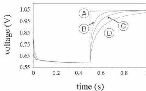
**Figure 6:** Cell voltage in response to a step change in the load.  $C_{dl}=0$  C (A), 0.5 C (B), 1 C (C), 2 C (D).
