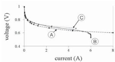
**Figure 8:** Polarization curves obtained assuming that: (A) the limit current is constant; (B) the limit current depends on the oxygen partial pressure; and (C) the exchange current does not depend on the limit current.
