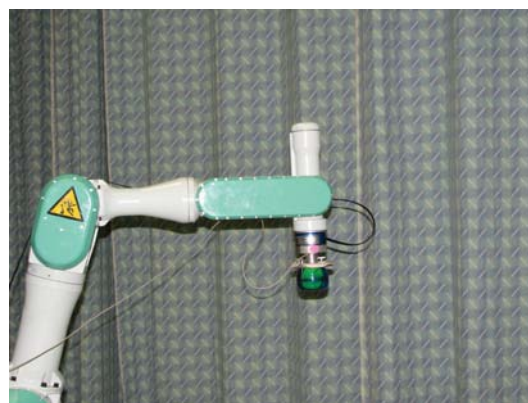
Figure 25: Experimental setup for spinning up the Power®Ball with PA10 robot
